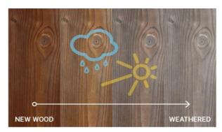
The Kebony technology gives the wood a deep rich brown colour (some natural colour variations will occur and there are possible darker areas as a result of the process). After exposure to sun and rain the wood will develop a natural silver-gray patina where surface cracks and checks may appear, this is a natural development and will not influence the performance and durability of the wood.
