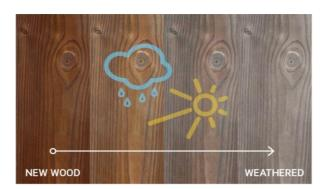
The Kebony technology gives the wood a deep rich brown colour (some natural colour variations will occur and there are possible darker areas as a result of the process). After exposure to sun and rain the wood will develop a natural silver-gray patina where surface cracks and checks may appear, this is a natural development and will not influence the performance and durability of the wood.
